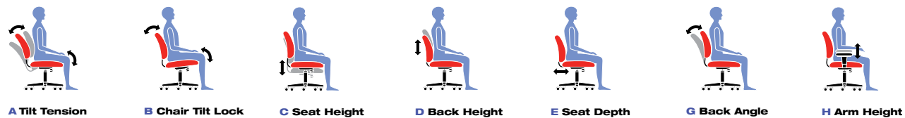
A Tilt Tension B Chair Tilt Lock C Seat Height D Back Height E Seat Depth G Back Angle H Arm Height
