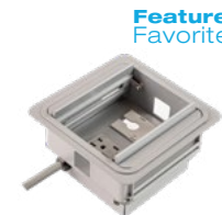
OTGPM-TUN Double door, recessed power block includes one duplex outlet, one USB-A port, one USB-C port and convenience duplex outlet underside of the unit. Field cut required, cutout template included. 7w x 7d x 4.972h List Price $635
