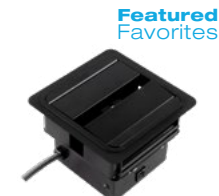
OTGPM-BLK Double door, recessed power block includes one duplex outlet, one USB-A port, one USB-C port and convenience duplex outlet underside of the unit. Field cut required, cutout template included. 7w x 7d x 4.972h List Price $635
