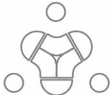
3-way layout Three curve-120 degree units, three half round units and three round units
