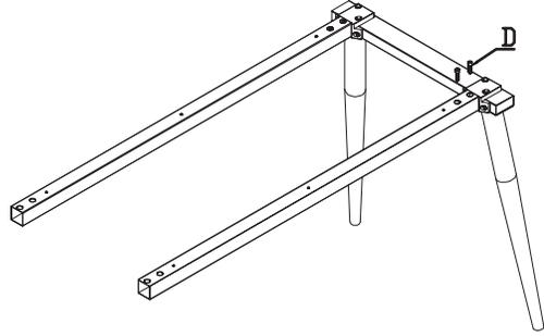
3. Install beam on Connector (A) with Screw (D)
