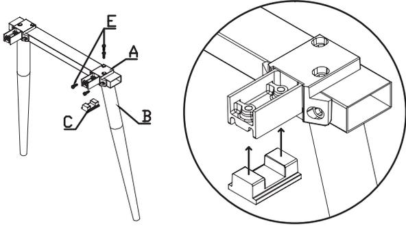
1. Install Connector (A) on Leg (B) with Screw (E)
