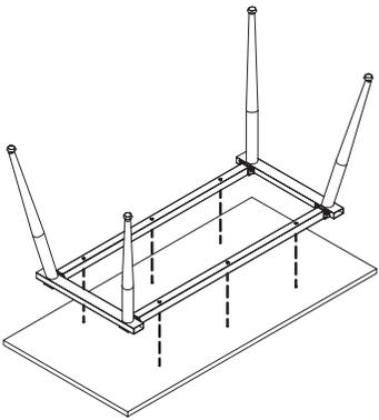
6. Align frame with pilot holes. Secure frame to top with wood screws provided with top surface
