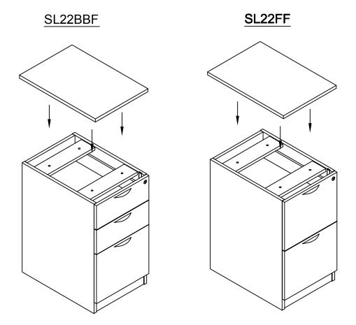
Use 4 M6\*40mm screws to attach top as provided with pedestal.
