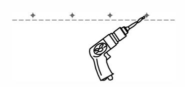
Care should be taken to mount the units. Units should be mounted to wall studs using correct fasteners. Failure to do so may result in collapse of the unit and subsequent personal injury. Mounting hardware not included. Mounting hardware used should be based on wall material. Consult an installation professional for proper wall mounting.
